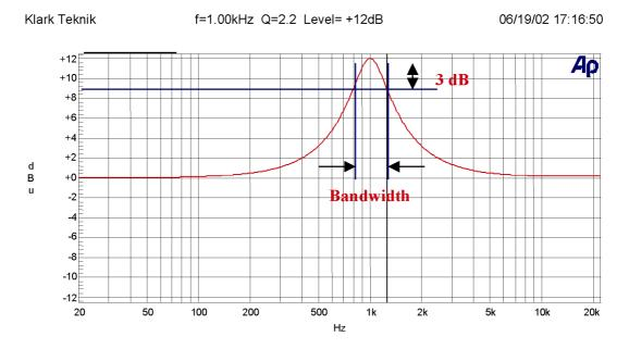
In the example above, the filter is centred on 1kHz, the lower 3dB point is at approximately 800Hz, and the upper one is at approximately 1.25kHz.
